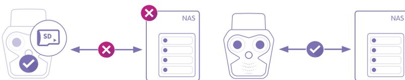
The microSD card fitted into every MOBOTIX camera is a backup storage device that continues to capture video recordings should the external network recording device fail (MxFFS Archive Storage). When reconnection is made, the camera will resync the recordings with the central recording device. No dedicated NVR or VMS is required to manage this fail-over process.
