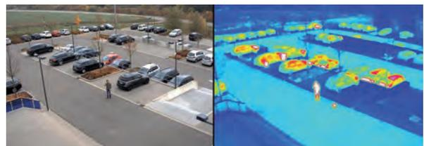
Combination of thermal and optical sensor, the most innovative dual camera system, embracing thermal, video and MxActivity sensor in one device to capture events in absolute darkness
